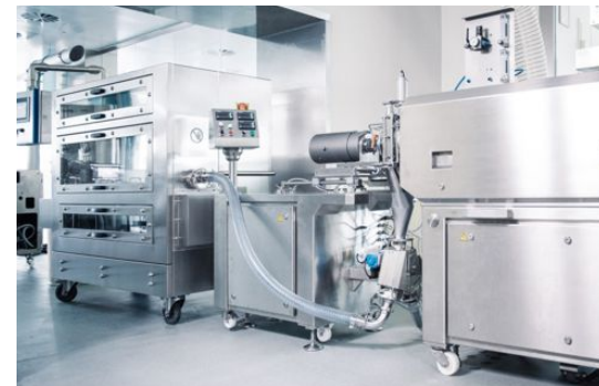
Figure 1: Commercial scale extrusion and pelletization process for manufacturing of INTAC ® IR pellets
